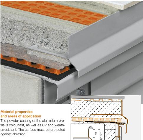
Penetrating water must not collect in the screed bed into which Schlüter®-BARA-RK has been anchored (installation of drainage layer), since water enriched with alkali will attack aluminium. In special cases, the suitability of Schlüter®-BARA-RK must be verified based on the anticipated chemical, mechanical, and/or other stresses.
