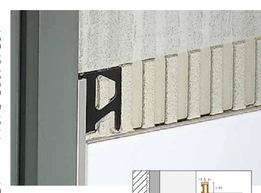
Schlüter®-DILEX-BWA is used in tile installations as a flexible connection to fixed structural components. Applications include window or door frames, thresholds, cupboard-wall connections, floor coverings against existing wall or dado coverings, etc.
