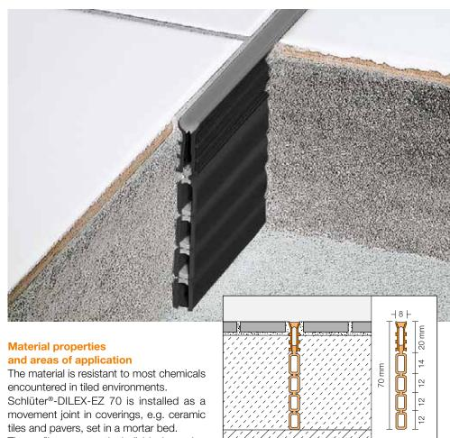
The profile separates the individual covering bays and neutralises compressive stresses in its centre section made of soft PVC. In special cases, the suitability of the profile must be verified based on the anticipated chemical, mechanical or other stresses.
